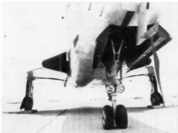
NOSE GEAR of Voodoo mounts twin landing lights, retracts forward. Note rugged structure of doors, needed to guarantee sealing under peak air loads of F-101's supersonic flight.
